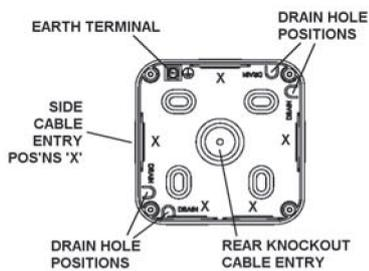
3. For cable entry, decide if conduit is being used & entry positions.
